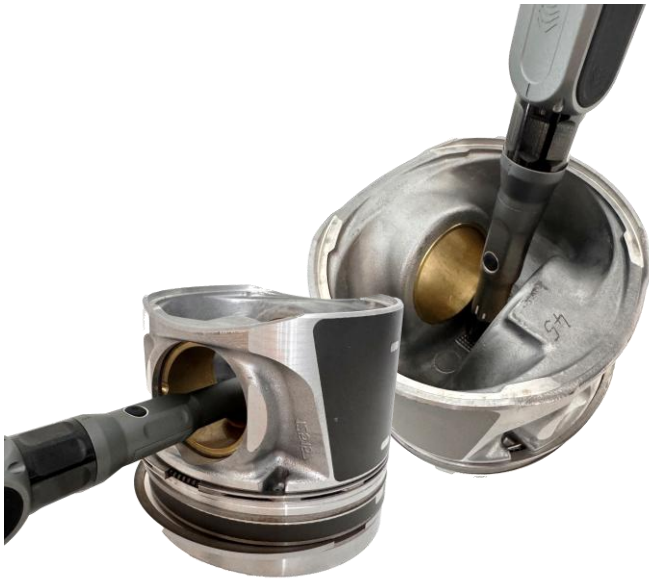
Figure 1: GelSight® Modulus™ straight and 90-degree lenses inspecting a piston
